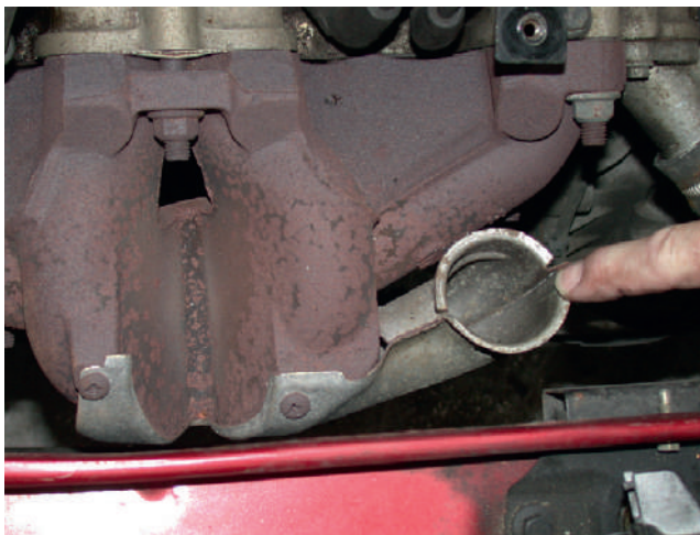
Figure 2.191 Pick-up for hot air on an exhaust manifold
